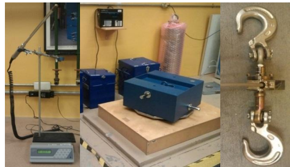
Data acquisition system, standard weight and load cell used in the calibration process.
