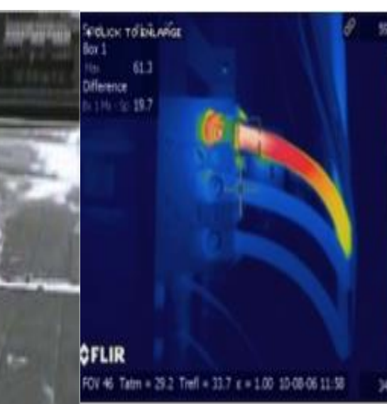
Loose connection on the top wire. (Infrared imaging services)
