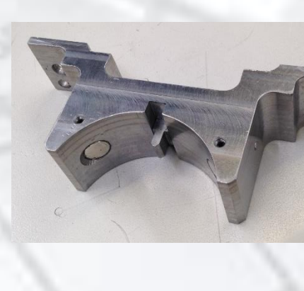
Figure 12: Armature support for station 3
