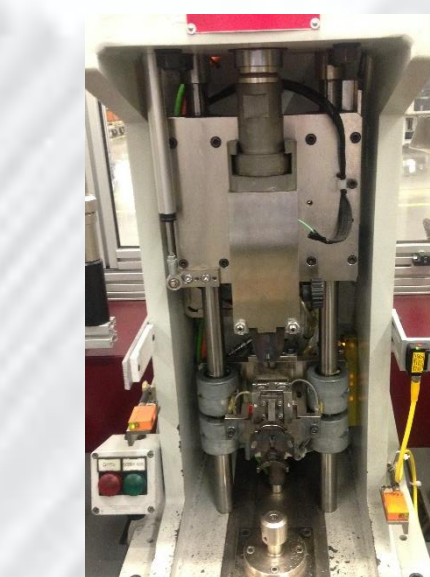
Figure 10: Commutator Press (Station 3)
