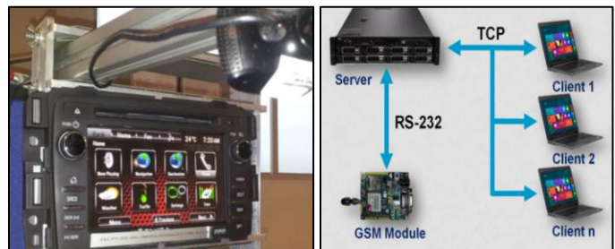
Infotainment system with camera for message verification and GEMA Structure
