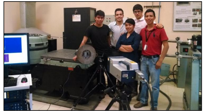
CENAM Team in the vibration laboratory conducting tests and modeling the brake disk for flexural and torsional vibrations
