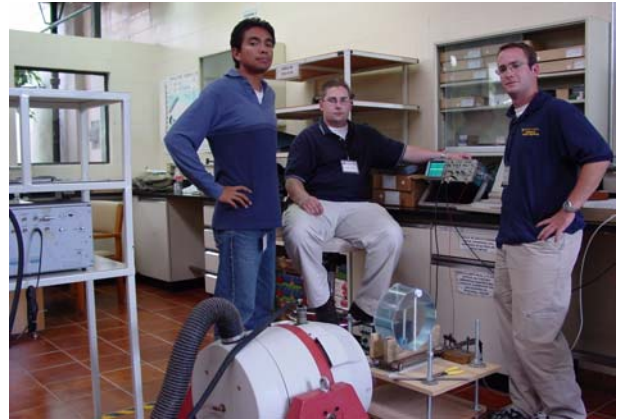
WVU-Queretaro students conducting experiments on the sloshing of a tank model
