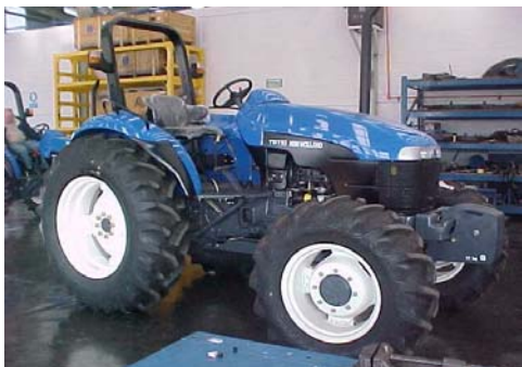
Tractor for which the ROPS is being designed
