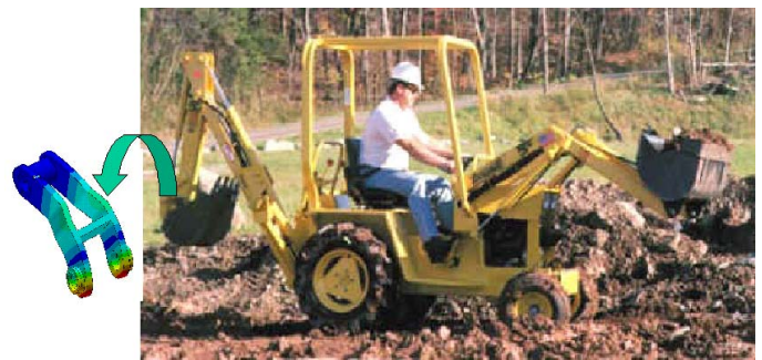
Compact construction equipment: Linkage finite element analysis for Terramite Corporation of WV
