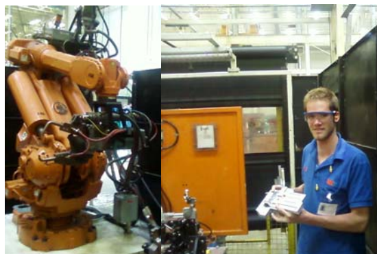
Welding robot for aluminum automotive structures
