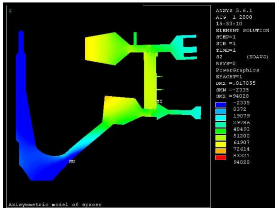
Axisymmetric model of a spacer with disks
