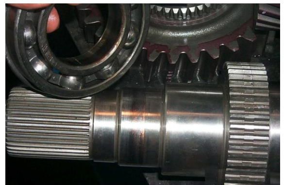
Gear and bearing elements of a heavy duty transmission
