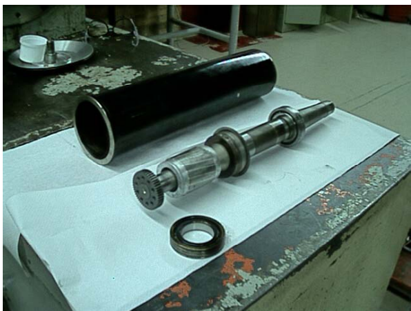
High speed rotor (godet) for polyester fiber production studies by the WVU-Queretaro team
