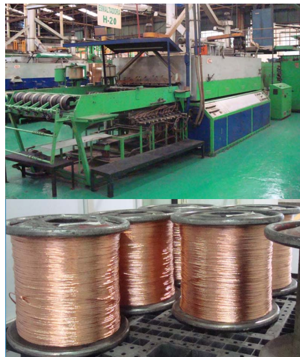
Magneto wire industrial oven in a Plant of the group ConduMex.
