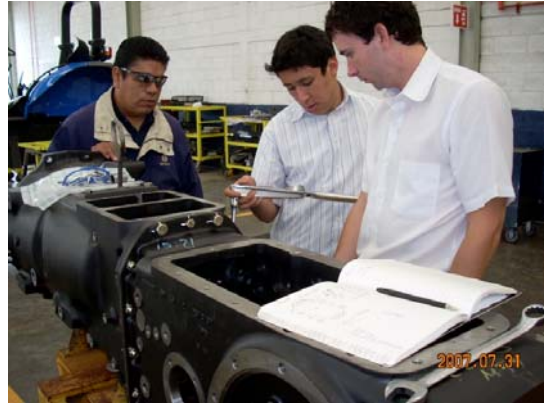
Luis (ITQ) and Richard (WVU) conducting torque tests with a technician at CNH
