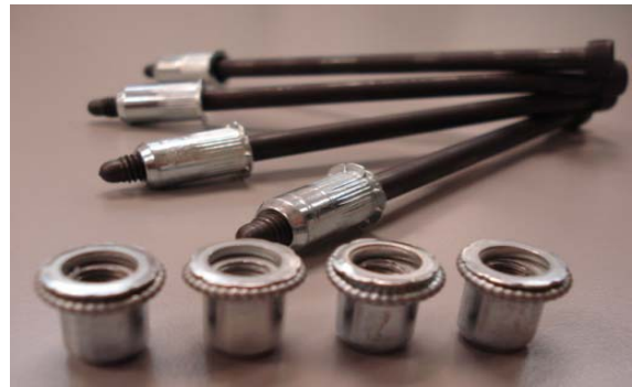
Rivnut and mandrel used to produce the rivet joint by direct pull through the threaded element.
